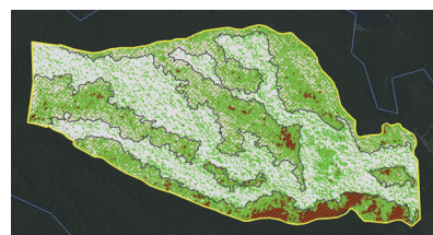
Fig. 1: Observations: Ground survey of burnt area (black line), overlaid on a burn severity assessment derived from RapidEye 5m satellite imagery (grey=unburnt, green=surface burnt, brown=surface burnt and canopy scorched).
